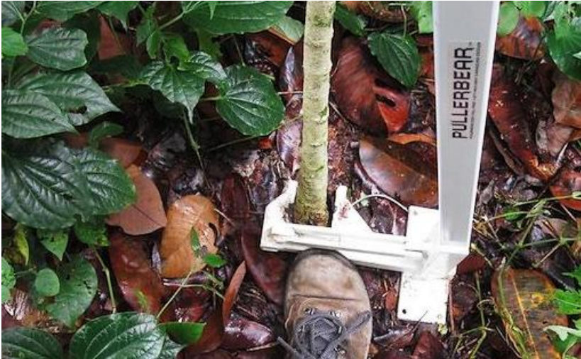
Fig. 3.2.1. Position the jaw of the Pulls-All tool around the base of the plant's stem using one's foot.
