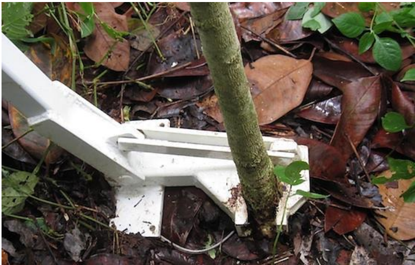
Fig. 3.2.2. When the handle is pulled, the jaws of the tool will bite into the stem's base.
