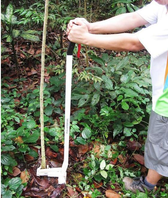
Fig. 3.2.3. Grab the handle of the tool with both arms and pull down to pull out the plant.
