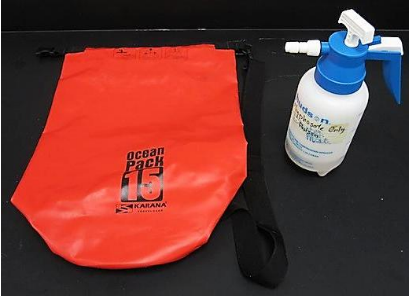
Fig. 4.1.1. Typical waterproof bag and pump-type sprayer available at most hardware shops and florists.
